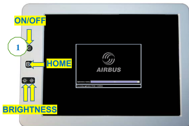
EFB G500 Smart Display Unit (SDU)
