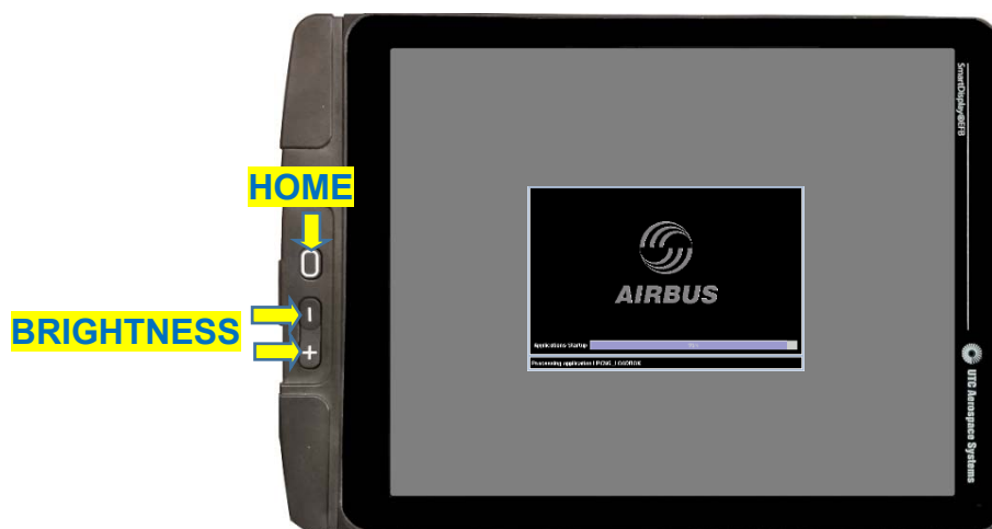
EFB G700 (UTC AEROSPACE) Smart Display Unit
